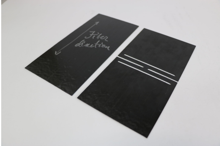
Figure 4.3: Unstrained LET joint With [90, 90, 0]_s ply schedule
