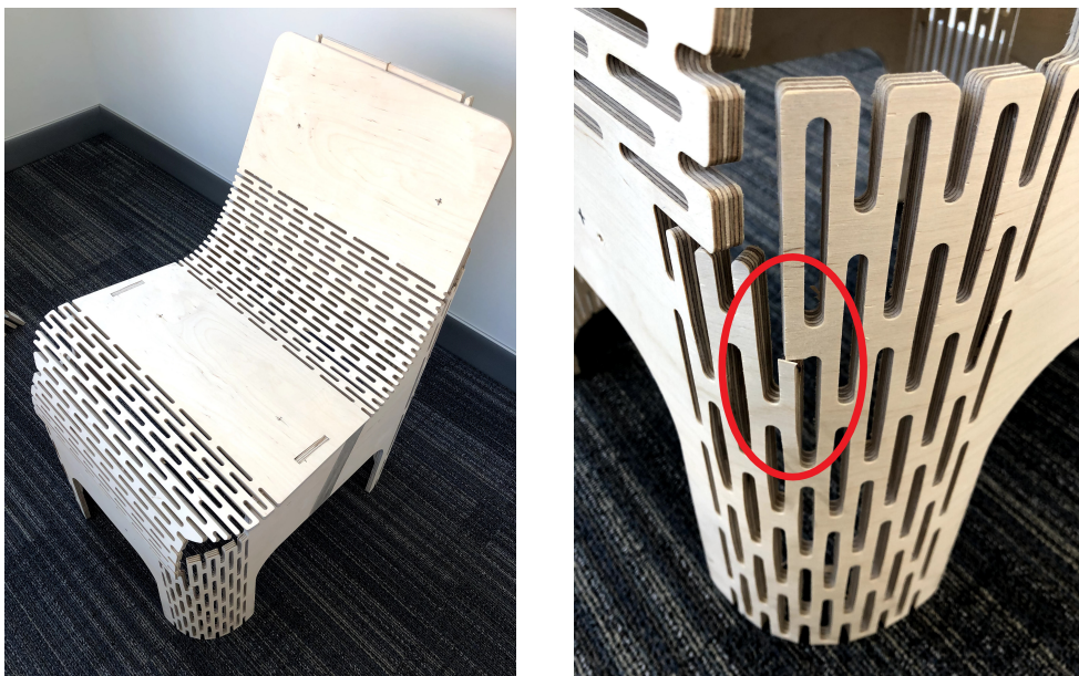
Figure 2.2: (Left) Plywood chair using LET arrays as hinges and (Right) broken torsional member in LET array
